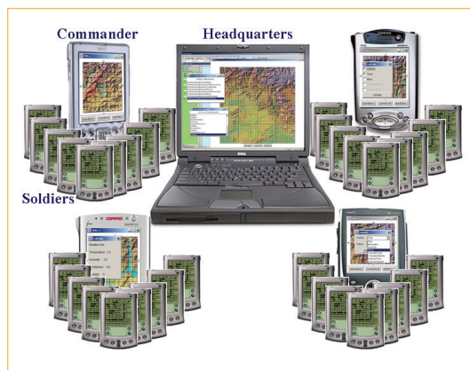
Figure 1. Troop deployment and battle simulations (TDS) application distributed across multiple devices. The headquarters computer is networked via secure links to a set of commander PDAs, which are connected directly to one another and to a large number of soldier PDAs.
